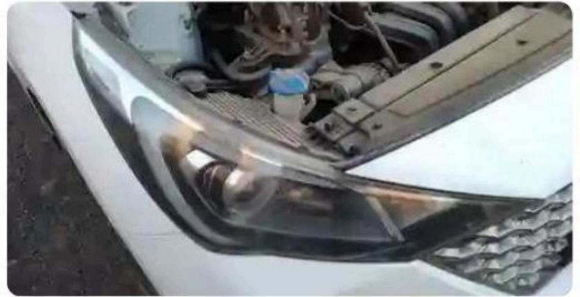
Light RHS Headlight: Scratched
