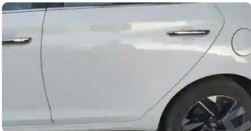
Door LHS Rear: No Dents, Repainted, Scratched
