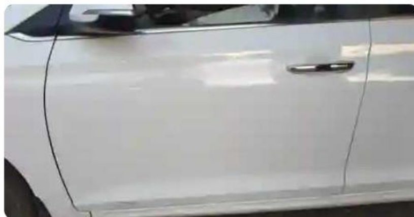
Door LHS Front: No Dents, Scratched, Repainted
