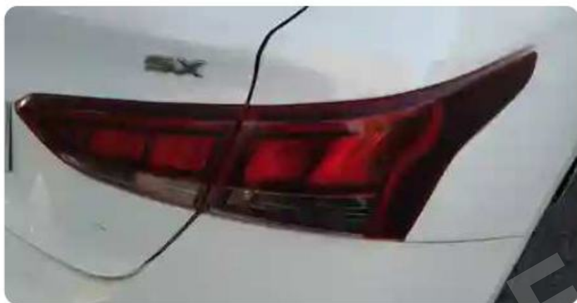
Light RHS Taillight: Scratched
