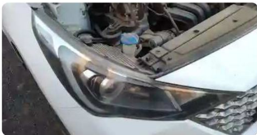
Light RHS Headlight: Scratched
